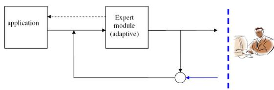
*A gold rule of the world of retroaction systems is that the retroaction measurement instrument has to be as exact as possible in order for the system to work well and react properly. Furthermore any error introduced in the retroaction is amplified in the loop*
